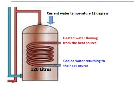
How much heat/energy in Kilojoules will it take to heat the cylinder above to 65°C. You must show your working out:
